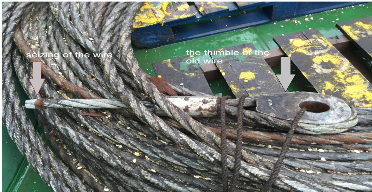
Figure 12: Seizing and cutting off the end of the crane cargo (hoist) old wire.
